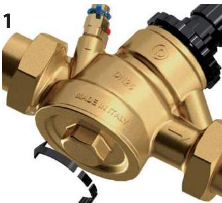
1 Unscrew bottom cap using a 30mm socket
